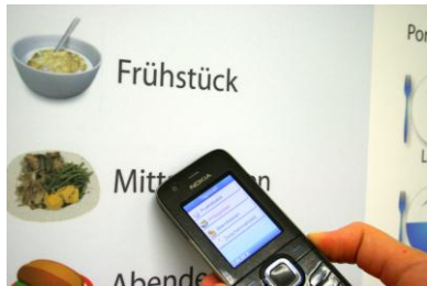
Figure 5. NFC phone on smartposter
